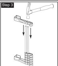
Place right hook on the end of the two tubes. Carefully line up and then firmly tap with hammer until they are completely in the sockets.
