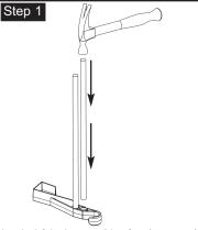
Lay the left hook on a solid surface (not carpet) with socket openings up. With a hammer, firmly tap one tube into each of the two sockets.
