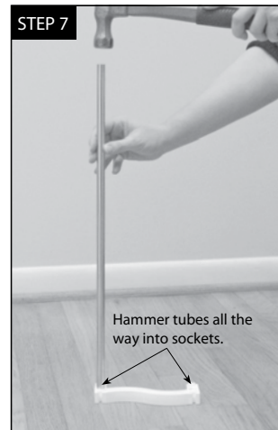
STEP 7: Assemble Connectors. Firmly hammer tubes into sockets.
